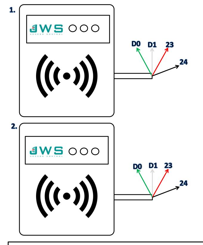
WHITE WIRES – PLACE INTO BLOCK WITH DIODE – THEN CONNECT TO D1
